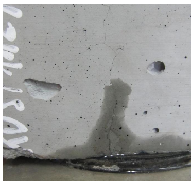
Figure 8. Water migrating through scratches in a specimen subject earlier to high temperature (own photo)
