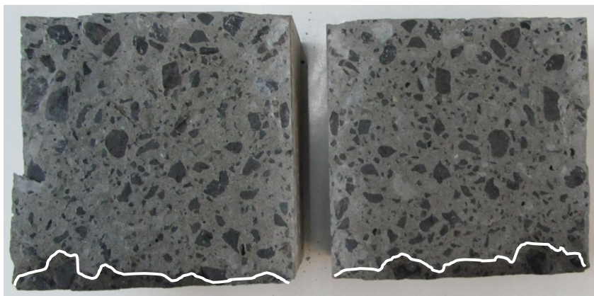
Figure 7. Wetted specimens of HPC comparative, non-exposed to high temperatures (own photo)
