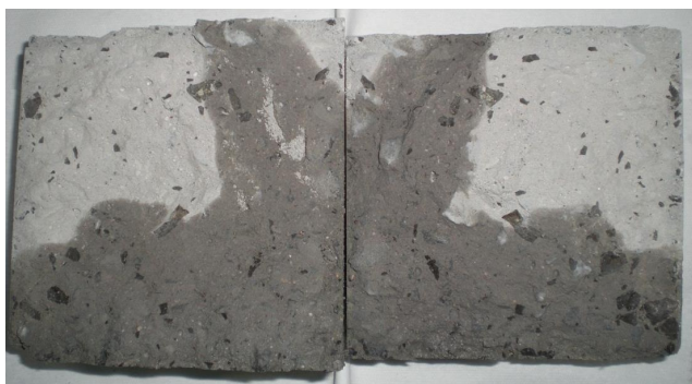
Figure 9. Specimen after water penetration depth study (after 600°C) (own photo)
