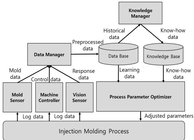
FIGURE 2. Data flow between functional modules
