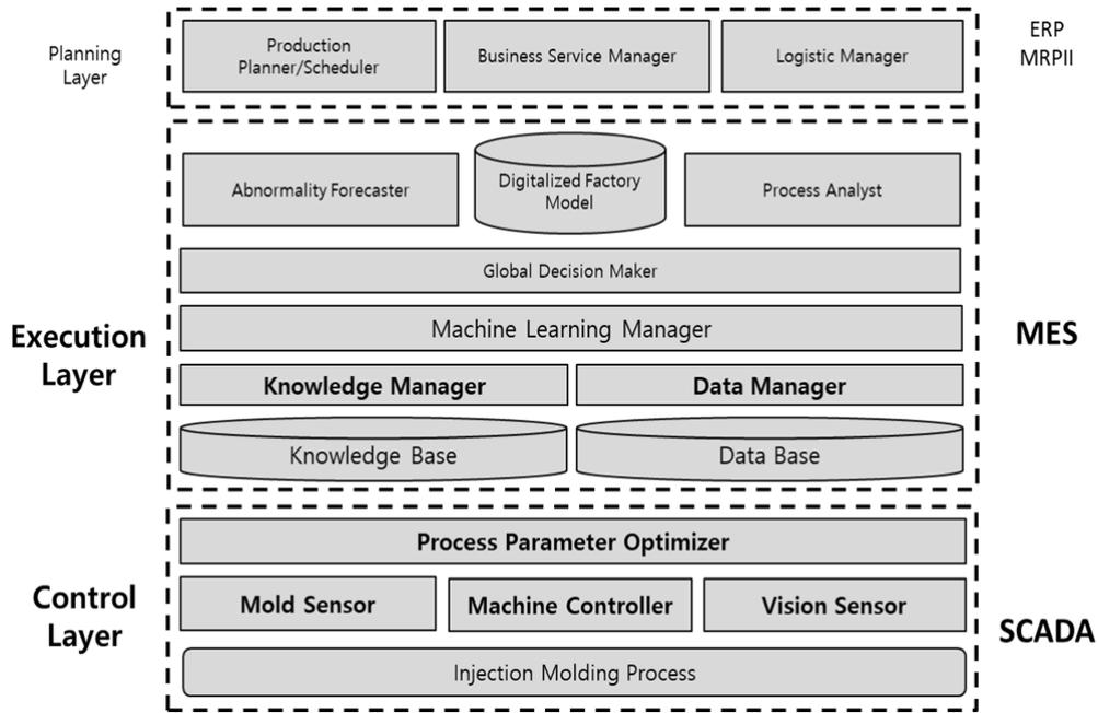
FIGURE 1. Framework of smart injection molding system
