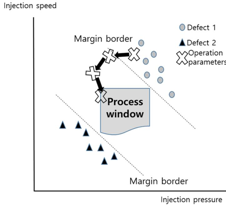
FIGURE 5. Process window for injection molding
