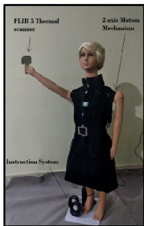
Figure 19: Humanoid Robot Model for Scanning with Thermal Camera
