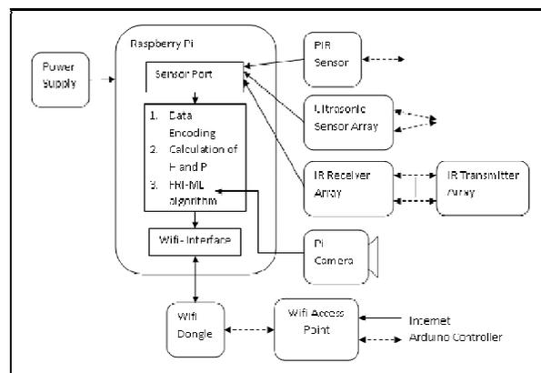
Figure 8: Entry Gate System using Raspberry Pi Controller
