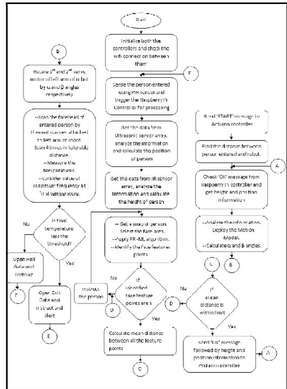
**Figure 2: Operational Flow Diagram of the Proposed System**
