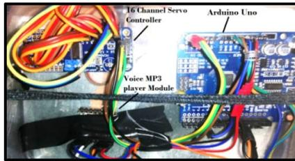
Figure 17: Arduino Controller with interfacings
