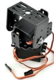
**Figure 9:** 2-axis Motion Mechanism
