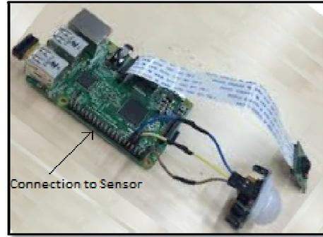
Figure 14: Raspberry Pi Controller for Entry Gate System
