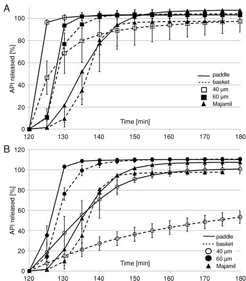
Figure 2. Release rate of diclofenac from loose MT 2 mm (A) and loose MT 3 mm (B) coated with 40 µm or 60 µm film thickness, in comparison with Majamil commercial tablets – the test performed in a paddle (solid line) and basket (dotted line) apparatus. These profiles were recorded in a buffer phase pH 6.8 following the acid phase.
