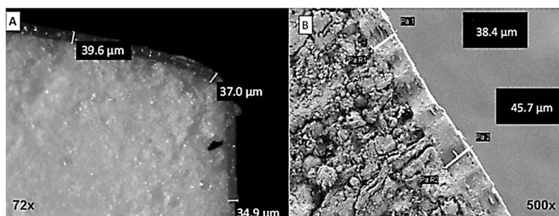
Figure 1. Stereoscopic microscope (A) and SEM (B) images of MT 3 mm/40  $\mu$ m cross-sections.
