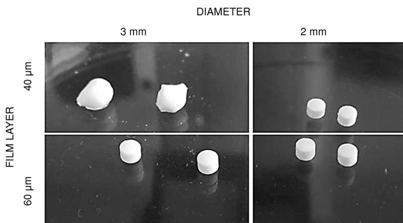
Figure 3. The image of enteric-coated MT after the acid phase of dissolution test (2 h in 0.1 M HCl).
