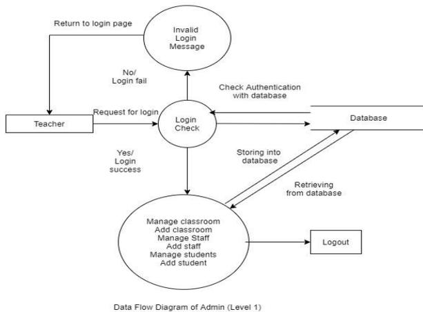
Fig 4. DATA FLOW DIAGRAM ( LVL 0 & LVL 1)
