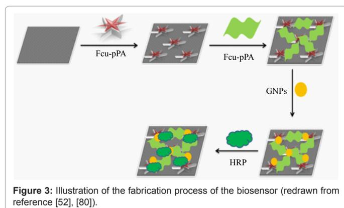
Figure 3: Illustration of the fabrication process of the biosensor (redrawn from reference [52], [80]).
