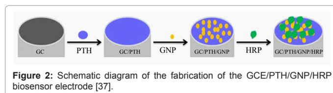
Figure 2: Schematic diagram of the fabrication of the GCE/PTH/GNP/HRP biosensor electrode [37].
