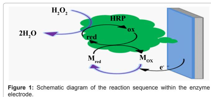
Figure 1: Schematic diagram of the reaction sequence within the enzyme electrode.
