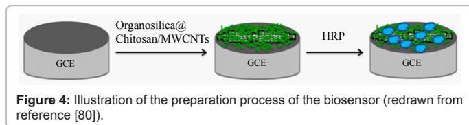
**Figure 4:** Illustration of the preparation process of the biosensor (redrawn from reference [80]).
