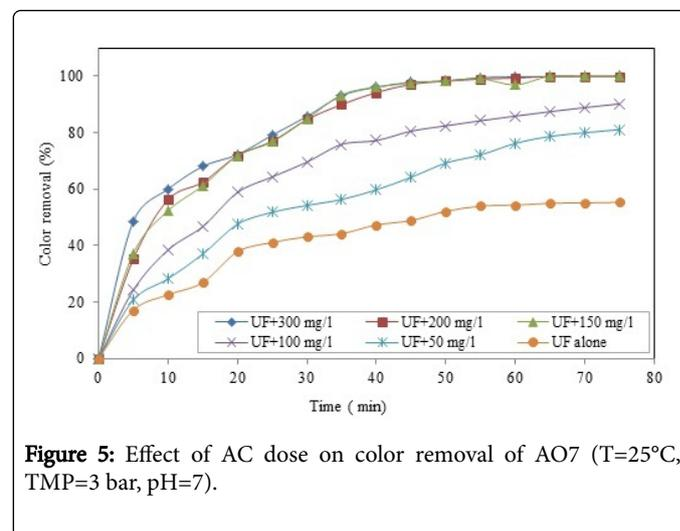
Figure 5: Effect of AC dose on color removal of AO7 ( $T=25^\circ\text{C}$ ,  $\text{TMP}=3 \text{ bar}$ ,  $\text{pH}=7$ ).
