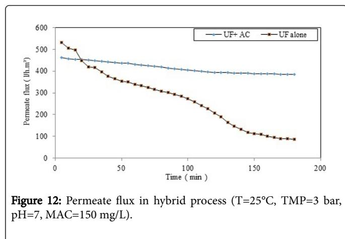
**Figure 12:** Permeate flux in hybrid process (T=25°C, TMP=3 bar, pH=7, MAC=150 mg/L).
