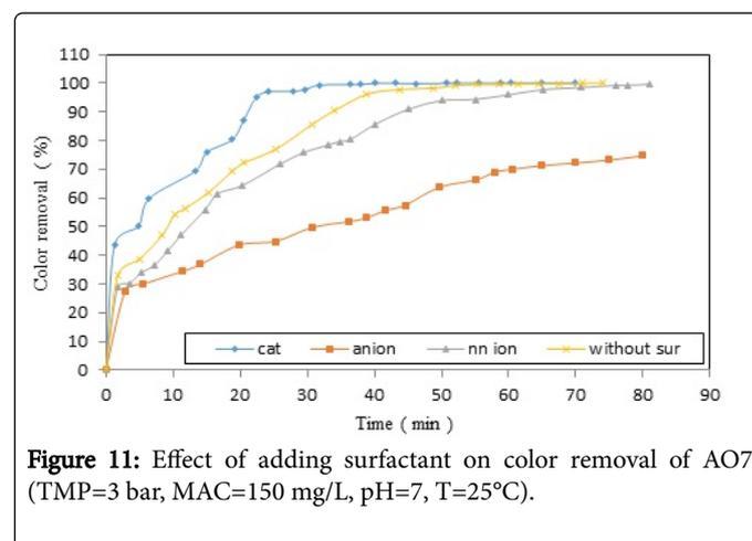
Figure 11: Effect of adding surfactant on color removal of AO7 (TMP=3 bar, MAC=150 mg/L, pH=7, T=25°C).
