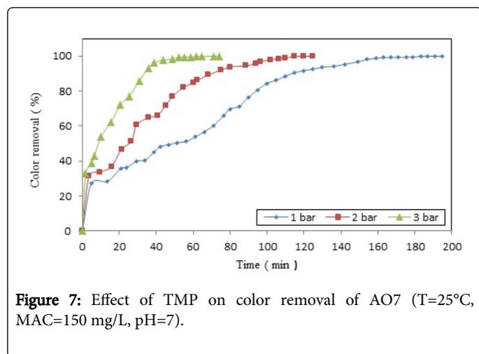
**Figure 7:** Effect of TMP on color removal of AO7 (T=25°C, MAC=150 mg/L, pH=7).
