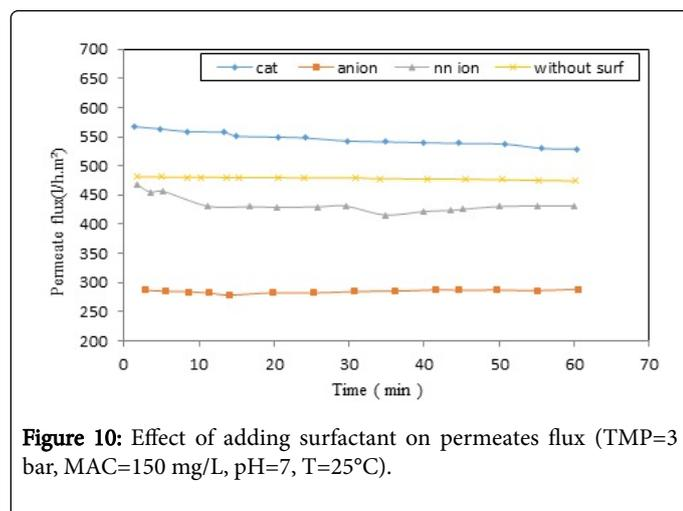
Figure 10: Effect of adding surfactant on permeates flux (TMP=3 bar, MAC=150 mg/L, pH=7, T=25°C).
