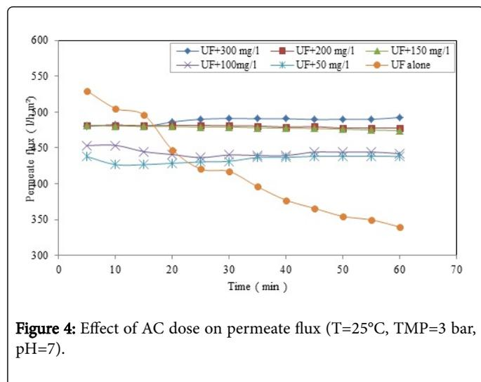
Figure 4: Effect of AC dose on permeate flux ( $T=25^\circ\text{C}$ ,  $\text{TMP}=3 \text{ bar}$ ,  $\text{pH}=7$ ).
