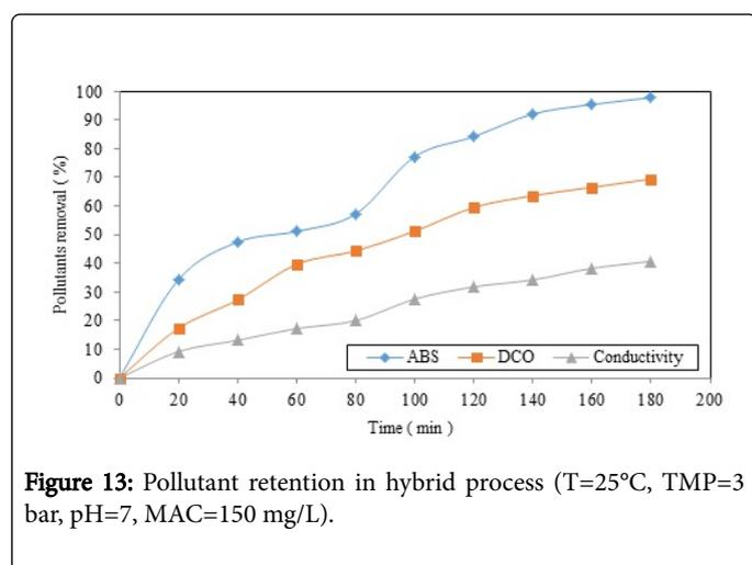
**Figure 13:** Pollutant retention in hybrid process (T=25°C, TMP=3 bar, pH=7, MAC=150 mg/L).
