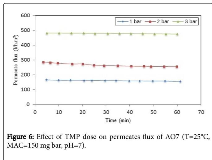
**Figure 6:** Effect of TMP dose on permeates flux of AO7 (T=25°C, MAC=150 mg bar, pH=7).
