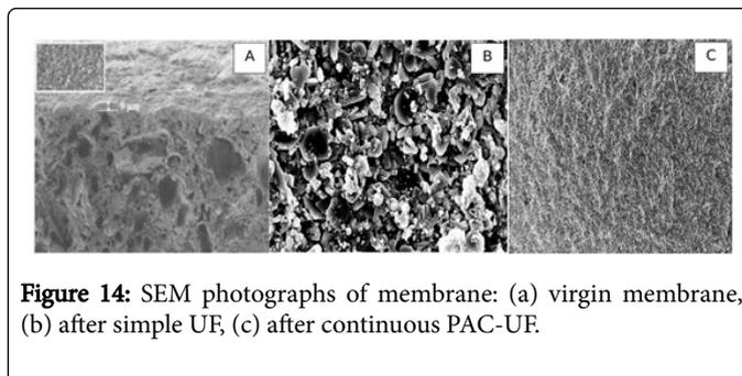
**Figure 14:** SEM photographs of membrane: (a) virgin membrane, (b) after simple UF, (c) after continuous PAC-UF.
