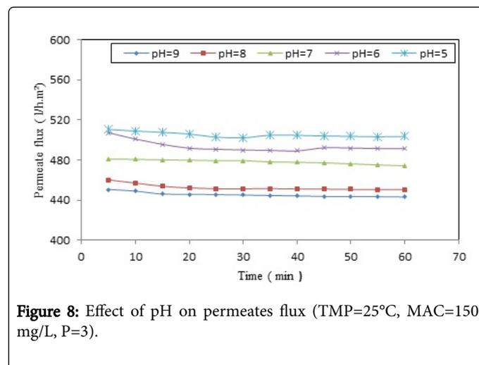
**Figure 8:** Effect of pH on permeates flux (TMP=25°C, MAC=150 mg/L, P=3).
