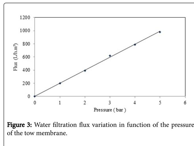
Figure 3: Water filtration flux variation in function of the pressure of the tow membrane.
