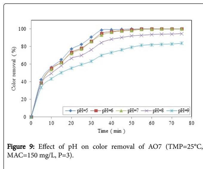
**Figure 9:** Effect of pH on color removal of AO7 (TMP=25°C, MAC=150 mg/L, P=3).
