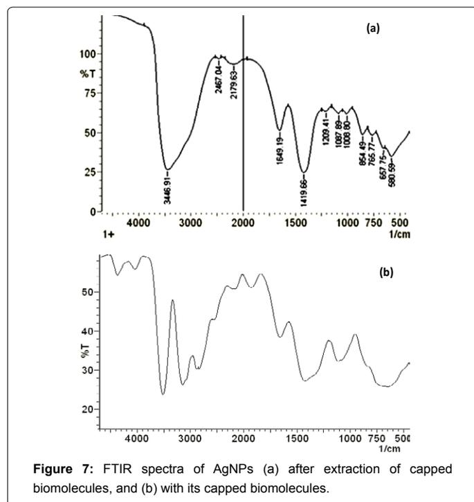
**Figure 7:** FTIR spectra of AgNPs (a) after extraction of capped biomolecules, and (b) with its capped biomolecules.
