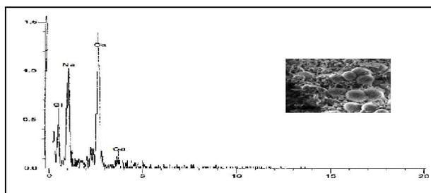
Fig.(6) EDX pattern and SEM photomicrograph of deteriorated limestone sample with fungal growth.
