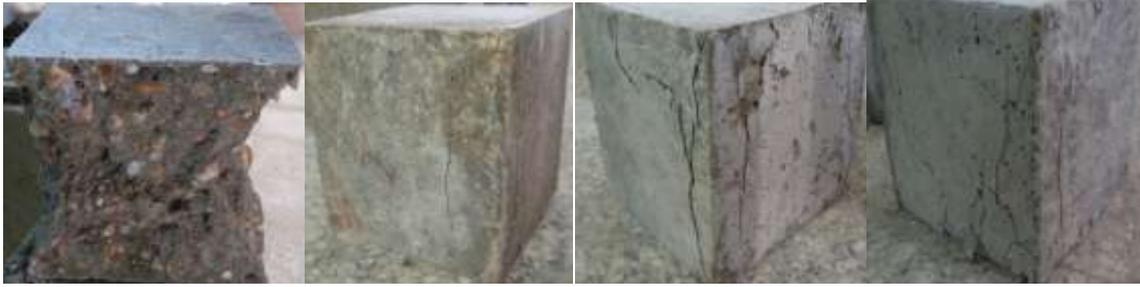
Figure 9: Failure Pattern of control and polypropylene fibre cubes under compressive strength test after 14 days.
