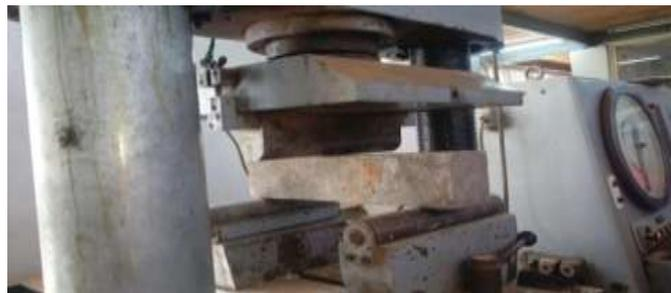
**Figure 3:** flexural strength test apparatus
