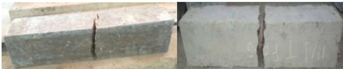
Figure 14: Failure Pattern of control and polypropylene fibre beam
