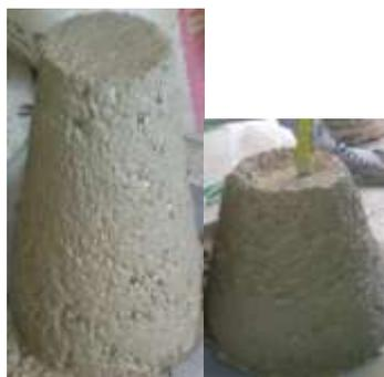
**Figure 6:** Slump tests for (i) polypropylene fibre without increase in super plasticizer dosages. (ii) Polypropylene fibre with increase in super plasticizer dosages.
