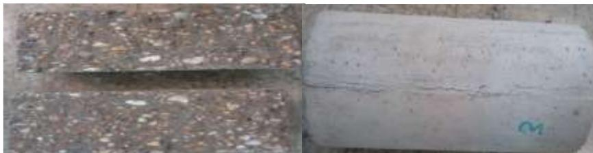
Figure 12: Failure Pattern of control and polypropylene fibre cylinders under the split tensile strength test.
